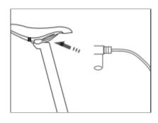
Charging port is on the upper right of the battery box , covered by a rubber dust-free cover, uncover it, plug the charger into the port; cover the port again when charged.
